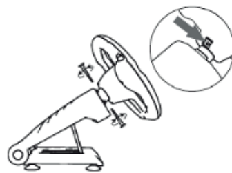
Secure the screws provided as shown with the included tool, do not overtighten.
